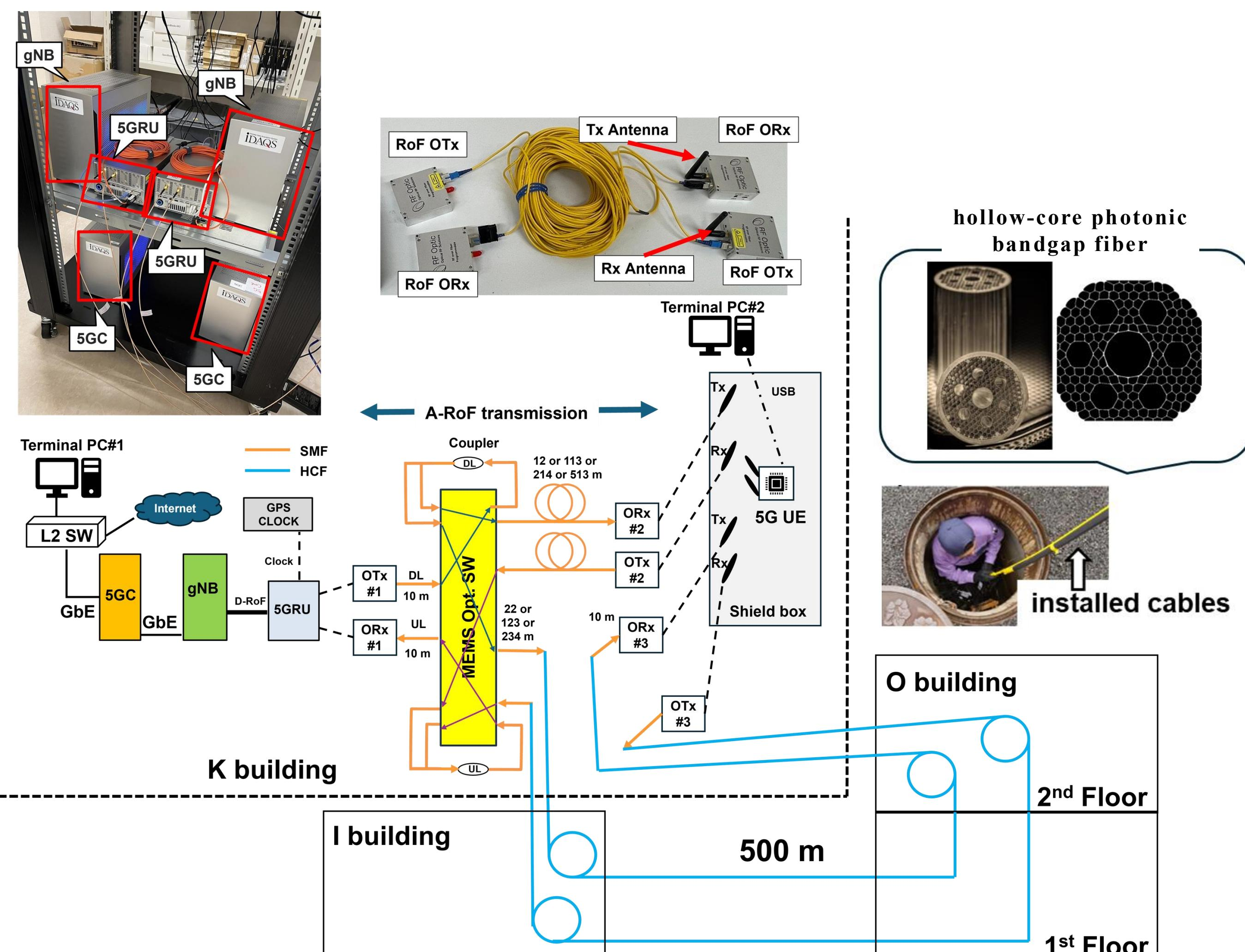
**A Sub6 analog RoF based local 5G system using a field installed hollow-core photonic bandgap fiber is constructed.**
