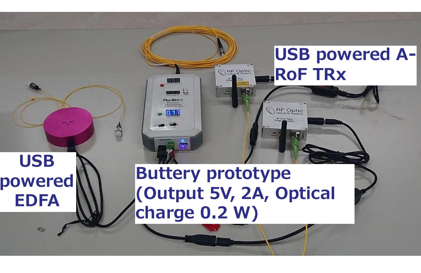
Optically charged buttify prototype and expected power supplied devices (EDFA, A-RoF TRx)
