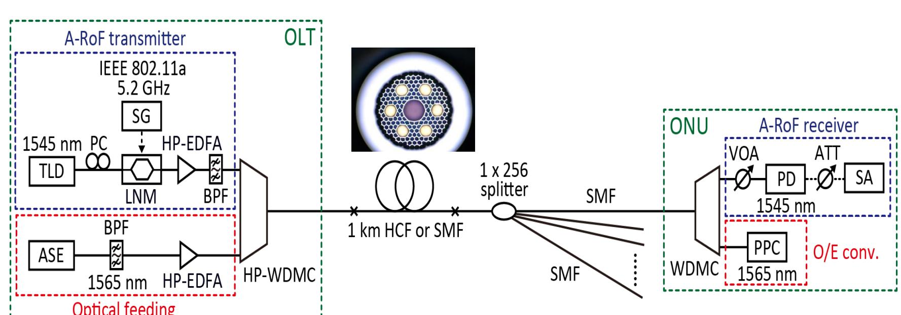
256 branches WiFi (5.2 GHz) signal transmission with optical power feeding
