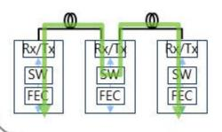
Separation of FEC from transmission frames enables the FEC signal processing to be optimized to the distance, and the intermediate FEC to be skipped.
