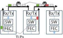
Burst traffic TLPs are set to the same length as fixed short size PLPs to minimize packet processing and buffering in SWs.
