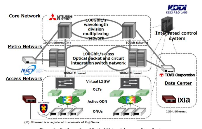
Figure 1 Configuration of Optical Network between Data Centers
