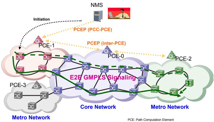
PCE: Path Computation Element PCC: Path Computation Client PCEP: Path Computation Element communication Protocol
